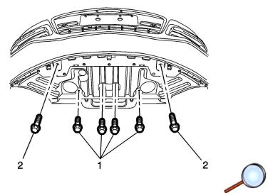
4. From under the vehicle, remove the 4 short fascia nappy bolts (1) and the 2 front long fascia support bolts (2).
