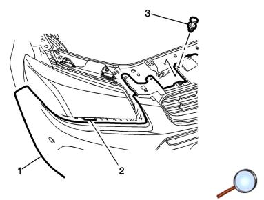
6. Remove the 2 scrivets (3) retaining the fascia to the front cross member. Carefully pull the fascia outwards to release the fascia from the fender retaining clips (1), then carefully pull the fascia forwards to release the fascia retaining clips (2) under the headlamps. Remove the vehicle fascia.
