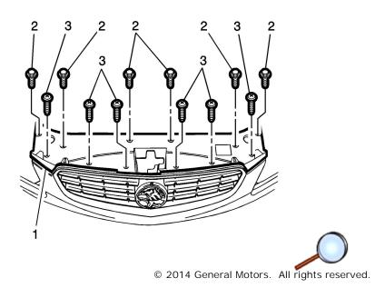
5. From under the vehicle bonnet, remove the 6 bolts (2) across the rear edge of the front fascia cover and the 6 screws (3) across the front of the front cover and remove the cover (1).
