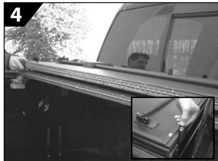
4 With the cover in the fully open and stacked position, secure all three docking straps. It is important to secure the docking straps at all times when the cover is in the fully open position.
