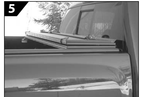
5 To close the cover, reverse these steps in the same order, making sure to close the rear panel last.
