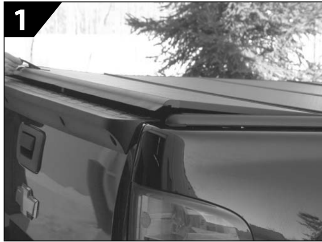
1 To open the cover lift the latch release handle and open the rear panel to the fully open position.
