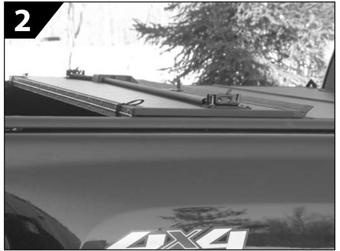
2 To insure proper operation of the center latch mechanism always open and fold the rear panel of the cover to its fully open position before starting any folding motion of the second or third panels.
